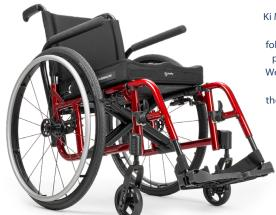
Ki Mobility's flagship product, the Catalyst 5 has since redefined the ultra-lightweight folding market by raising the bar in weight, performance, durability and functionality. Weighing in at 23 lbs and constructed from ultra-lightweight 7000 series aluminum, the Catalyst 5 is arguably the best choice in high-performance folding wheelchairs.
